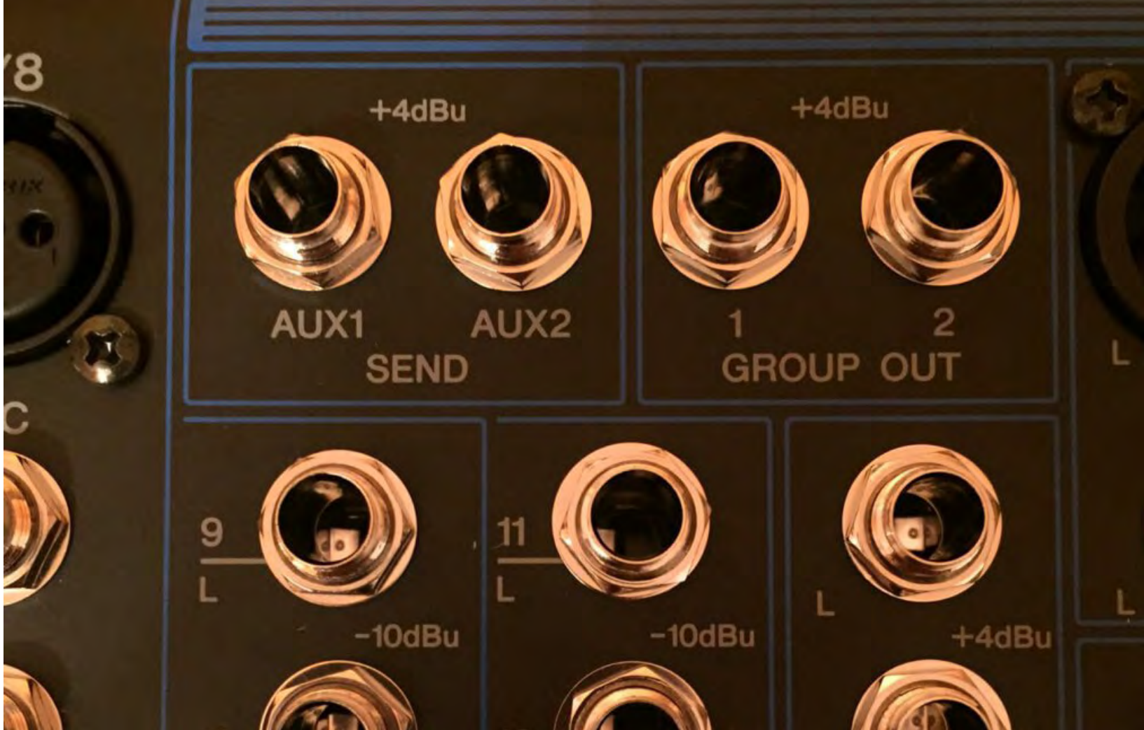
above: the output section of your mixer will allow you to route audio from the unit to auxiliary equipment
